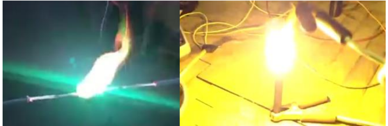
DC fault arcing due to loose terminals (simulation)
